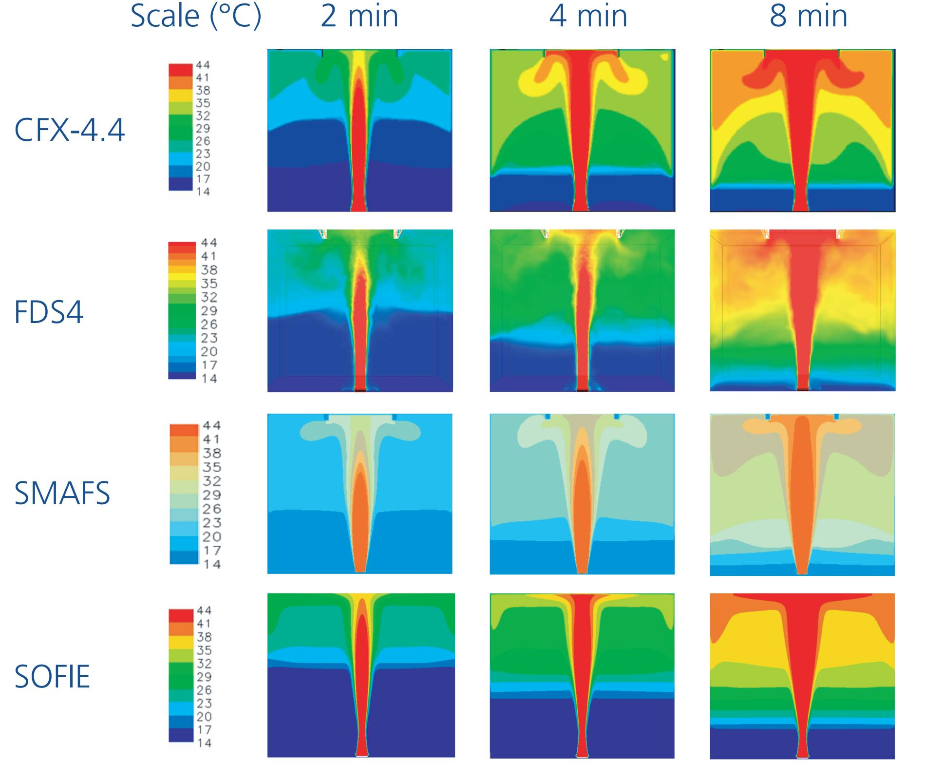
NOTE: The comparison between the codes shows strong influence of geometry aspects. The comparison with the experiment (see diagram on the right) shows different accuracies (e.g. smoke layer height and temperature) for the different codes.
